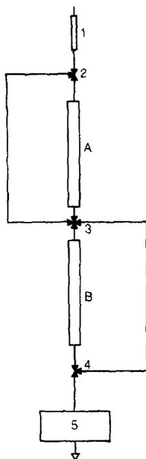
Fig. 1. Coupled system with pre-column (1) and separation columns (A) and (B); 2, 3, 4, valves; 5, refractive index detector.
