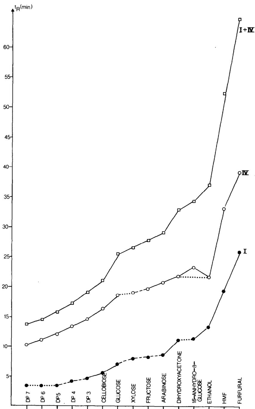
Fig. 3. Dependence of retention time,  $t_R$  (min), on the use of single and coupled columns (I and IV) for the investigated substances. —, Good resolution; - - -, minimum loss of resolution; ·····, no resolution. Chromatographic conditions as in Fig. 2.
