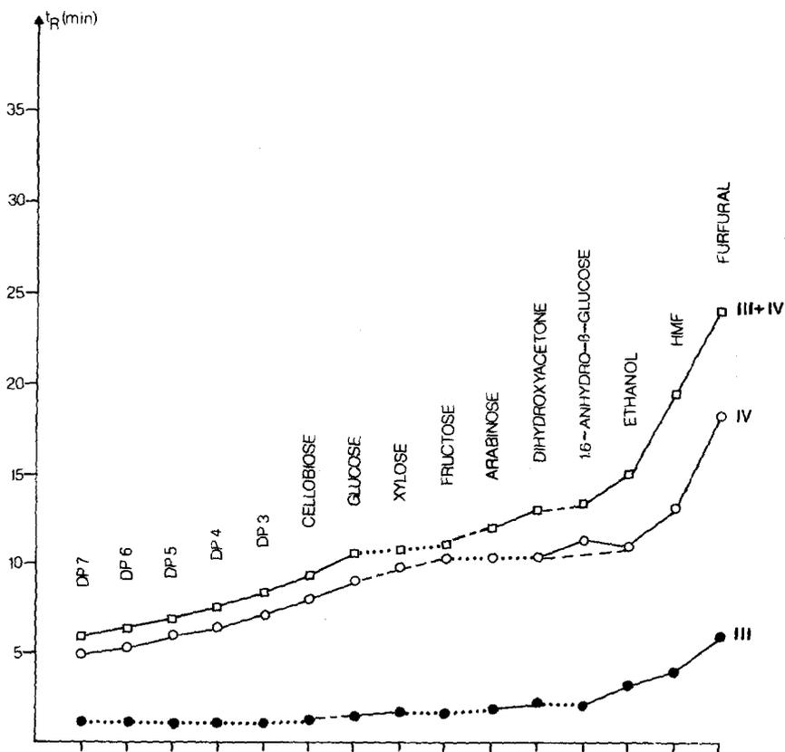
Fig. 9. Dependence of retention time,  $t_R$  (min), on the use of single and coupled columns (III and IV) for the investigated substances. —, Good resolution; - - -, minimum loss of resolution; ·····, no resolution. Chromatographic conditions as in Fig. 8.
