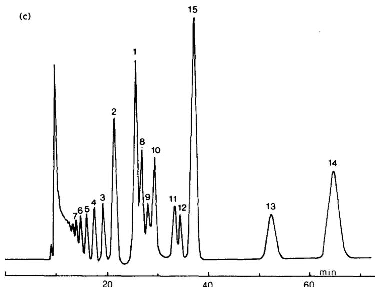
Fig. 2. Optimized separations of a standard mixture. For peak identification, see Table I. Chromatographic conditions: column temperature, 85°C; mobile phase, water; flow-rate, 0.6 ml/min; refractive index detection. Column: (a) I; (b) IV; (c) coupled I + IV.
