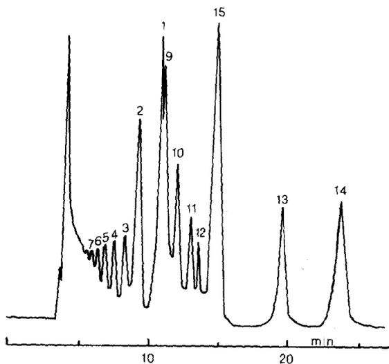
Fig. 8. Optimized separation of a standard mixture. For peak identification, see Table I. Chromatographic conditions: coupled columns III + IV; column temperature, 95°C; mobile phase, water; flow-rate, 1.2 ml/min; refractive index detection.
