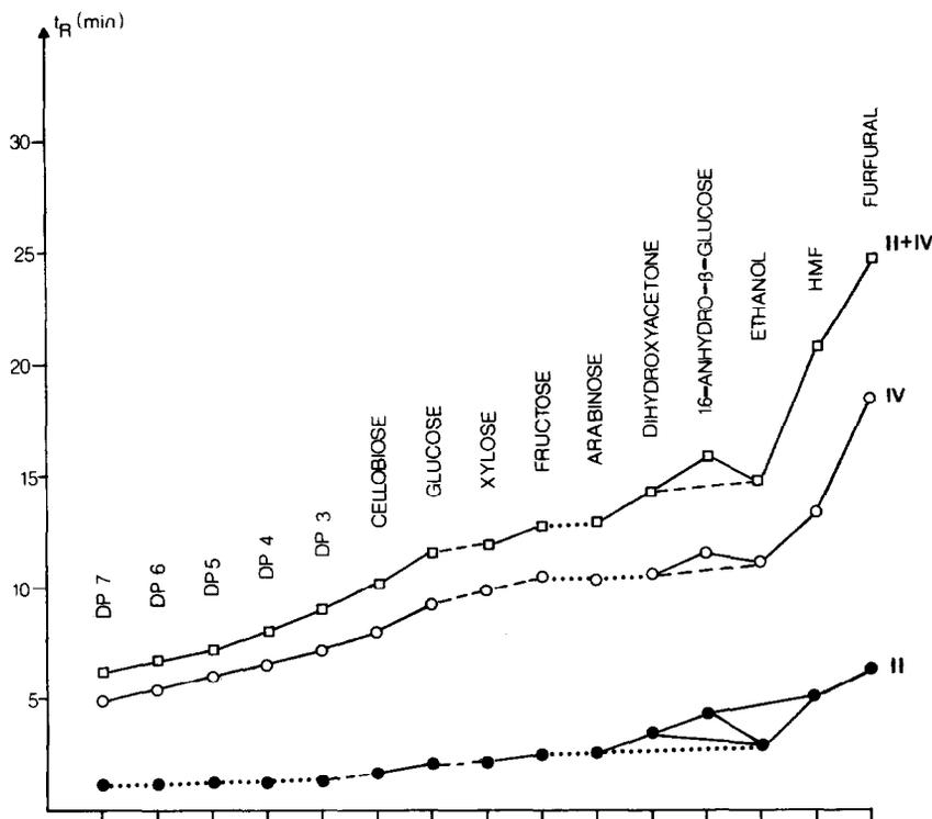
Fig. 7. Dependence of retention time,  $t_R$  (min), on the use of single and coupled columns (II and IV) for the investigated substances. —, Good resolution; ---, minimum loss of resolution; ·····, no resolution. Chromatographic conditions as in Fig. 6.
