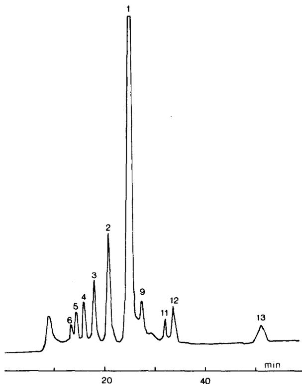
Fig. 10. HPLC trace of a hydrothermally degraded poplar wood sample. Conditions as in Fig. 2. For peak identification, see Table I.
