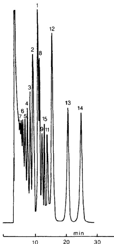
Fig. 6. Optimized separation of a standard mixture. For peak identification, see Table I. Chromatographic conditions: coupled columns II + IV; column temperature, 95°C; mobile phase, water; flow-rate, 1.2 ml/min; refractive index detection.
