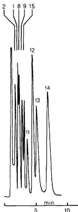
Fig. 5. Optimized separation of a standard mixture. For peak identification, see Table I. Chromatographic conditions: column, II; column temperature, 95°C; mobile phase, water; flow-rate, 1.2 ml/min; refractive index detection.
