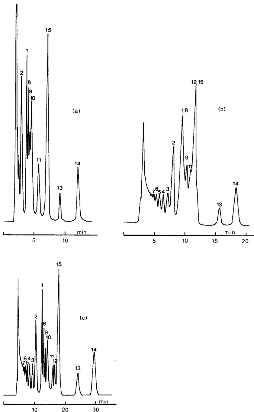
Fig. 4. Optimized separations of a standard mixture. For peak identification, see Table I. Chromatographic conditions: column temperature, 95°C; mobile phase, water; flow-rate, 1.2 ml/min; refractive index detection. Column: (a) I; (b) IV; (c) coupled I + IV.
